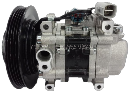
DENSO CAT NO. 44-106 COMPRESSOR TYPE: TV12C (R134A) CAR MODEL: COROLLA 1.6L YEAR MODEL: 1997 GROOVE: 4PK
