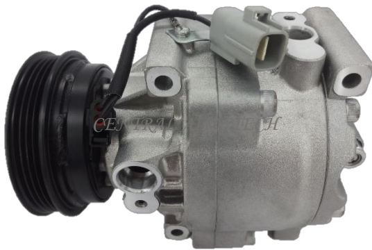
DENSO CAT NO. 44-045 COMPRESSOR TYPE: SC08C CAR MODEL: PASEO/TERCEL 1.5L YEAR MODEL: 1998 GROOVE: 4PK
