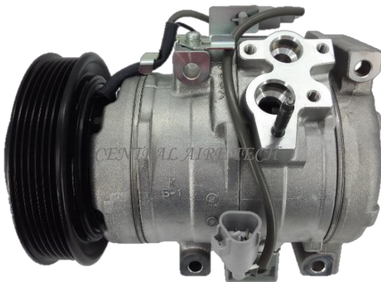
DENSO CAT NO. 44-142 COMPRESSOR TYPE: 10S17C (98 ohms) CAR MODEL: WYNDHAM/MARK YEAR MODEL: GROOVE: 6PK
