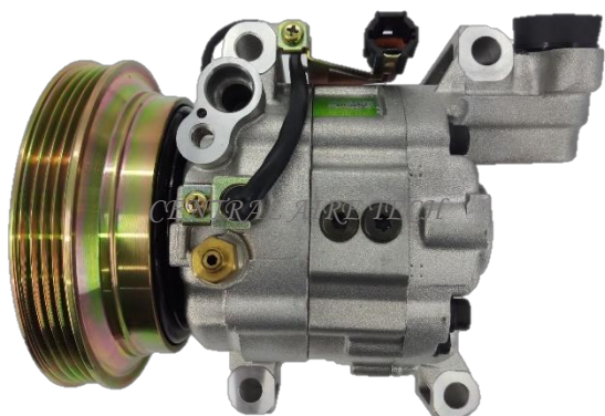
ZEXEL CAT NO. 32-131 COMPRESSOR TYPE: DKV11G CAR MODEL: SENTRA GX YEAR MODEL: GROOVE: 4PK
