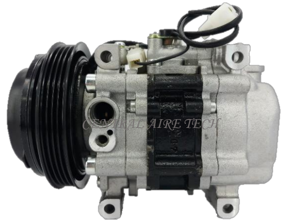
DENSO CAT NO. 28-040 COMPRESSOR TYPE: TV12C (R12) CAR MODEL: MIATA 1.8L YEAR MODEL: 1994 GROOVE: 4PK
