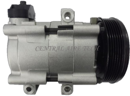
HALLA CAT NO. 14-086 COMPRESSOR TYPE: FS10 (3DM) CAR MODEL : F150 YEAR MODEL: GROOVE: 6PK
