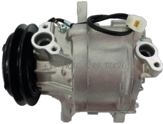
DENSO CAT NO. 11-007 COMPRESSOR TYPE: SC06E (3EM RSF) CAR MODEL: CUORE L700S YEAR MODEL: 1998-2005 GROOVE: 1A
