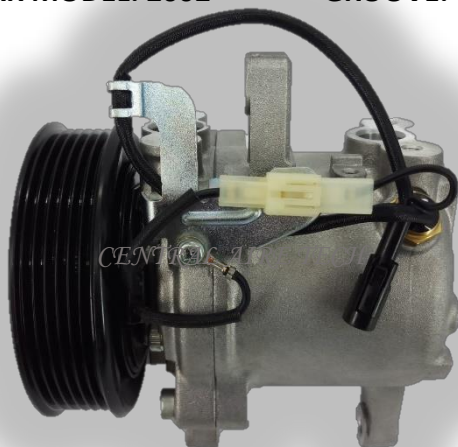
DENSO CAT NO. 11-005 COMPRESSOR TYPE: SV07E (3EM) CAR MODEL: CHARADE YEAR MODEL: GROOVE: 6PK
