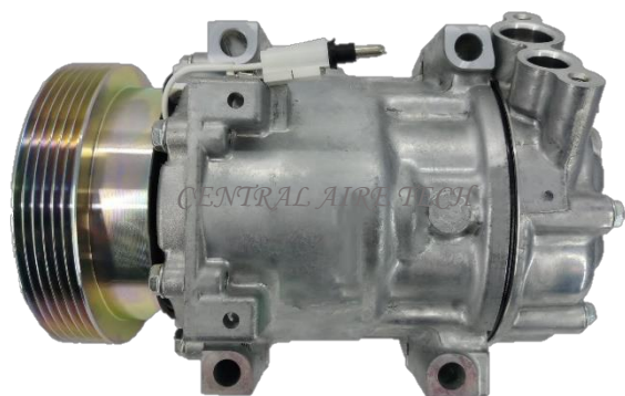
SANDEN CAT NO. 10-006 COMPRESSOR TYPE: SD7V16 (VPP) CAR MODEL: DUSTER YEAR MODEL: 2010-2018 GROOVE: 6PK
