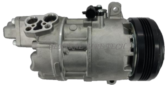
CALSONIC CAT NO. 02-022 COMPRESSOR TYPE: CSV613 (LSF) CAR MODEL: E46 YEAR MODEL: GROOVE: 4PK
