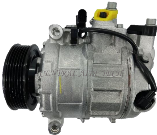
DENSO CAT NO. 45-033 COMPRESSOR TYPE: 7SEU17C CAR MODEL: PHAETON 3.0TDI YEAR MODEL: 2004-2008 GROOVE: 6PK
