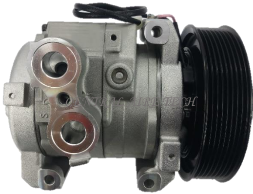
DENSO CAT NO. 29-049 COMPRESSOR TYPE: 10S15C CAR MODEL: ACTROS 24V YEAR MODEL: GROOVE: 8PK
