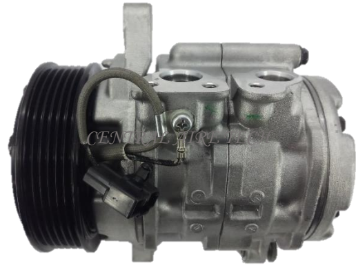
DENSO CAT NO. 44-096 COMPRESSOR TYPE: 10S11E CAR MODEL: AVANZA 1.5L YEAR MODEL: 2003-2008 GROOVE: 6PK
