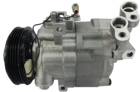
ZEXEL CAT NO. 43-016 COMPRESSOR TYPE: DKV08R CAR MODEL: SWIFT/SPLASH 1.2L YEAR MODEL: 2008 GROOVE: 4PK
