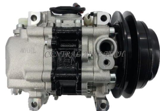
DENSO CAT NO. 22-098 COMPRESSOR TYPE: TV12C (LSF) CAR MODEL: ELF (12V) YEAR MODEL: 1999 GROOVE: 1A
