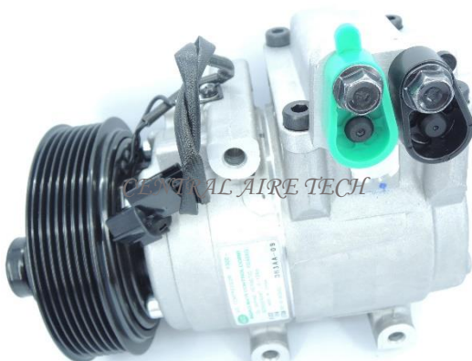
HALLA CAT NO. 20-053 COMPRESSOR TYPE: HS15 CAR MODEL: PORTER 2.5L DSL YEAR MODEL: 2013-2014 GROOVE: 7PK
