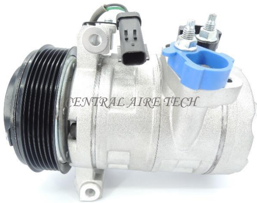
VALEO CAT NO. 12-009 COMPRESSOR TYPE: DKS17DS (RSF) CAR MODEL: NITRO/JEEP WRANGLER 3.8 YEAR MODEL: 2007-2011 GROOVE: 6PK
