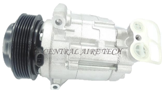
DELPHI CAT NO. 07-035 COMPRESSOR TYPE: CSP17 (3DM) CAR MODEL: TRAILBLAZER YEAR MODEL: 2012 GROOVE: 6PK
